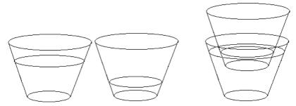
**Explanation of why the cups worked together to set the "water line" to where it started when just the one cup was full** (note, it's a little technical and maybe not needed): This is a vivid example that floating objects are buoyed up with a force equal to the weight of the water that they displace. Since the disposable tumblers are nearly weightless compared to the water that we are working with, the weight of the floating object is equal to the weight of water it contains.
